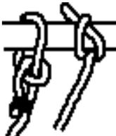
This is the capsized overhand knot. It is very useful to carry light loads, which have to be removed easily. Ashley recommends it to use it for hanging store to out of reach for mice. It should not be disturbed.
