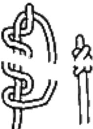
If you make more than two turns in the overhand knot it will be fatter. (But hardly stronger.) In twined rope it is important to work up the knot very carefully. (It will not only look neater, it will prevent 'kinking' which will weaken the rope even more!)
