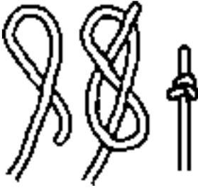
This knot is larger, stronger and easier to untie than the overhand knot. It does not harm your rope as much as the overhand knot does. So therefore sailors use this knot in most cases. (! not for bend support, where the smaller overhand is used, or in rope, a permanent small stopper)
