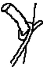
It is used to attach rope to a belay-pin, a weaver needle or even to a tree branch, to start belaying, to start winding or as a temporary easy to spill made-fast.
