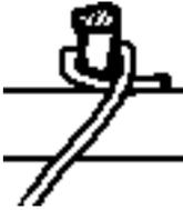
Although this is probably the simplest knot of all, you have to be a skilled knot-tier to know how to tie and use it in a safe way. The loose end of the rope is nipped against the object and the standing part. The best nip is obtained against an edge or shoulder. If the load is released and the standing part shaken, the hitch is spilled
